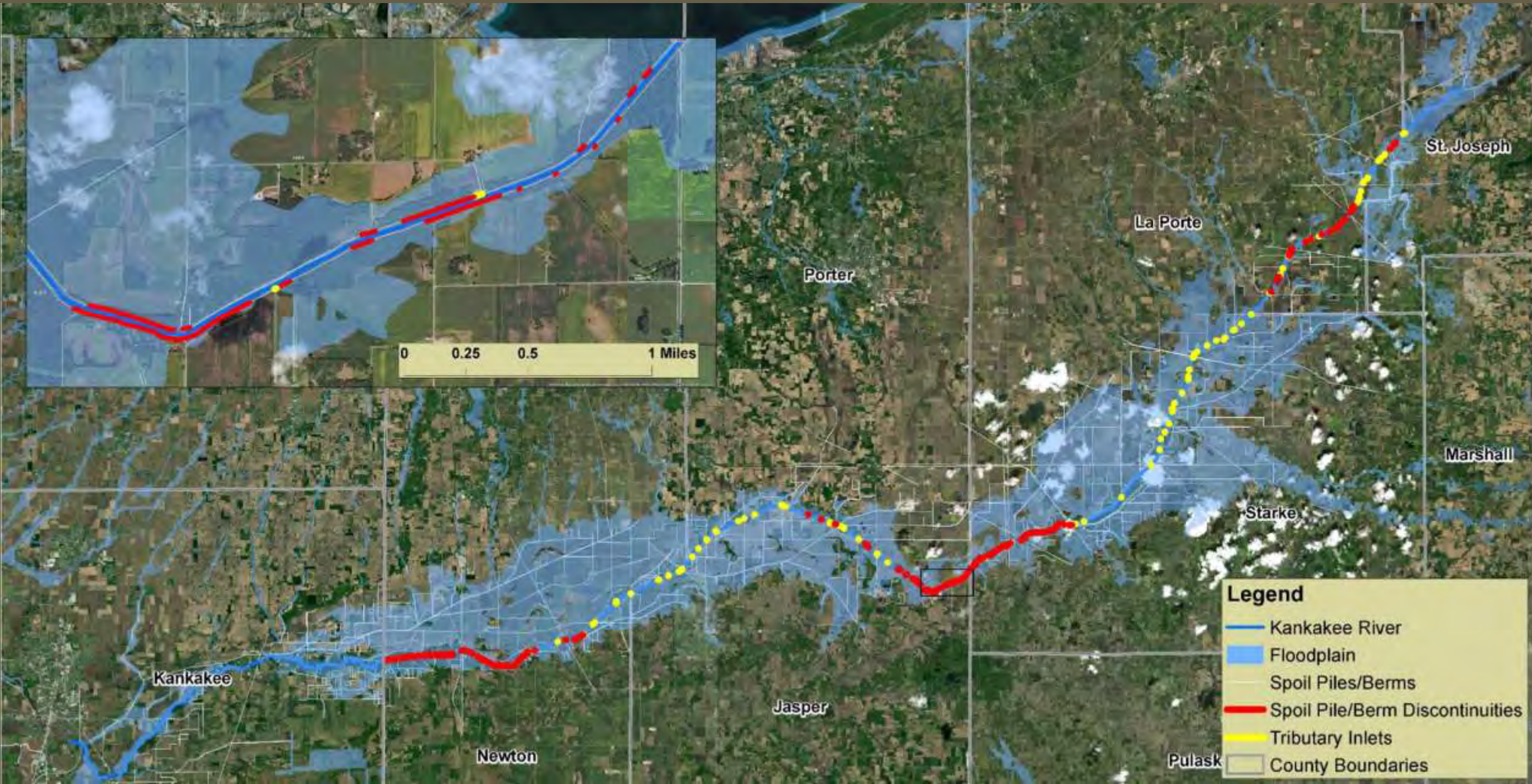
Berm discontinuities along Kankakee River
