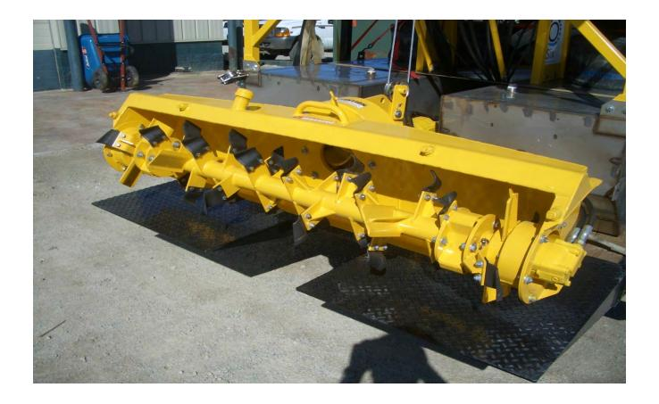
A pump is mounted to a pipe with a spinning head on the end. The pipe is lowered to the bottom and the cutter head feeds material and water to the pump.
